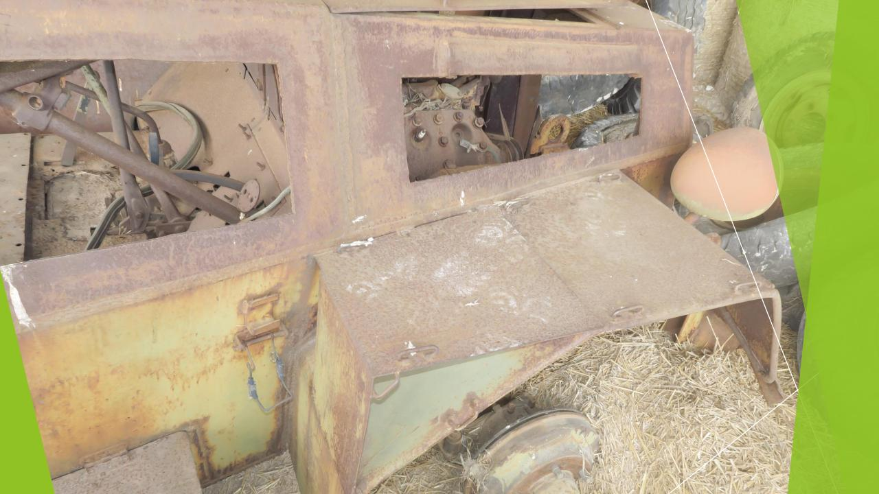
We still face several challenges. Completion of the upper superstructure will prove a challenge but what is fortunate is that the superstructure is a skeleton of angle iron and flat bar (the frame) to which the armour plate is fixed to form the armoured hull. The existing angles provide the most difficult structural answers. Due to no known survivors of this early Marmon Herrington Mk III, there may well have difficulties in checking exact physical details.
